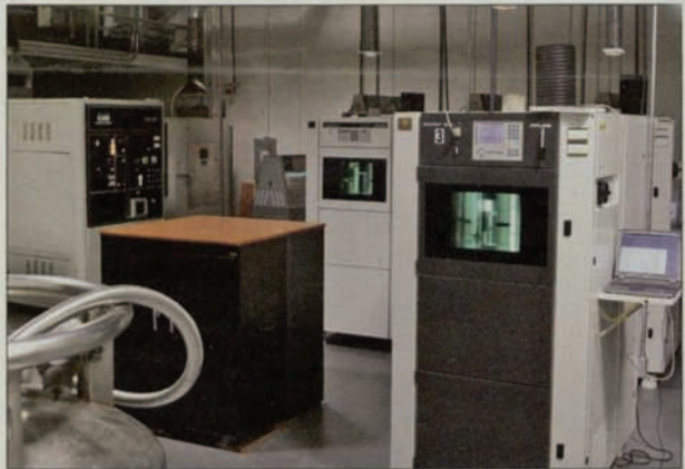
Americhem's weathering lab allows researchers to test the firm's outdoor materials under varying exposures to sunlight, heat and water.
