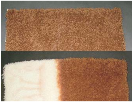
Fig. 5 Effect of bleach on solution dyed (top) and space dyed (bottom) PA carpet samples
