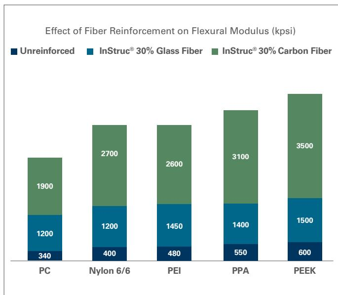
Flexural modulus improves by up to 6x with 30% carbon fiber reinforcement compared to unfilled base resins.
