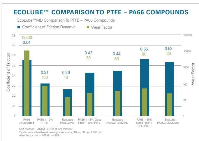
EcoLube™ PA66 grades deliver the same improvements in wear resistance and reduced friction as PTFE-filled nylons, without PFAS. These internally lubricated compounds extend part life, reduce noise, and eliminate the need for external lubricants in sliding and moving components.
