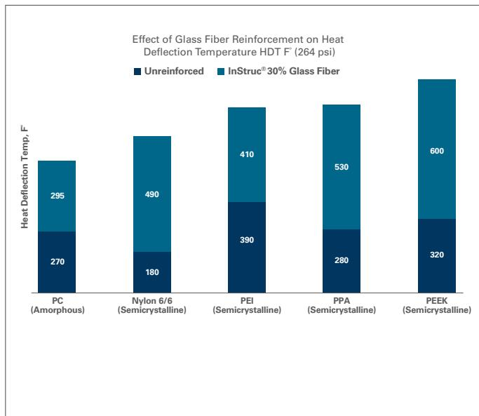
Glass fiber reinforcement improves heat deflection temperature (HDT) by up to 2.5x over unfilled base resins, with the largest gains observed in semicrystalline polymers.
