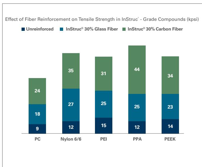
InStruc® compounds are formulated with glass or carbon fiber to deliver lightweight, high-strength materials that can replace metal in demanding applications.
