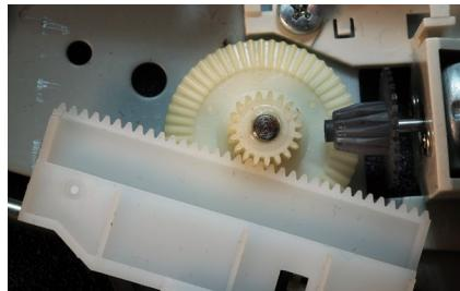
**InLube™ Wear-Resistant and Internally Lubricated Compounds:** Internally lubricated compounds for low friction and high wear resistance for increased service life, reduced noise, and maximum durability. PFAS-free alternatives to standard PTFE-containing wear and friction packages.
