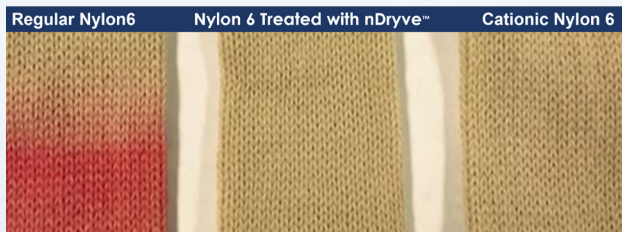
Untreated nylon shows visible stain penetration, while nDryve™-modified fibers maintain reduced surface staining.
