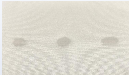
Control PET Fabric: No Water Repellency; Complete wetting observed
