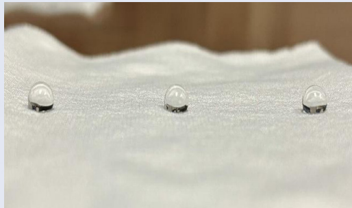
PET Fabric + nDryve™ Hydrophobic: Improved hydrophobic behavior with visible water beading
