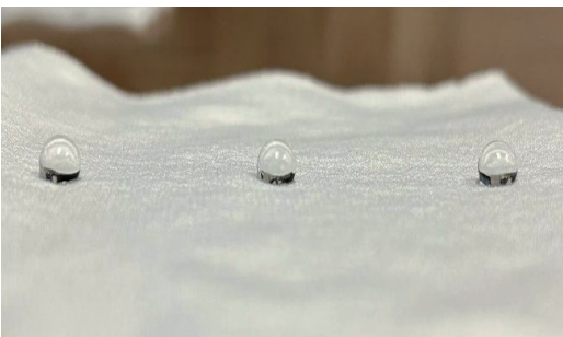
PET Fabric + nDryve™ Hydrophobic: Improved hydrophobic behavior with visible water beading
